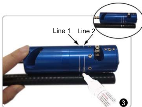
Align the end of cable with the end of trimming tool and make two marks on the cable jacket that correspond with lines 1 and 2 on the trimming tool.
