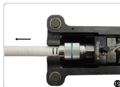
19 Press the trigger on the compression gun until it cycles and you hear a "pop". Do not pull or push on compression gun during compression.
