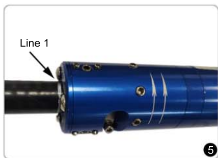
Insert the cable into the trimming tool. Select the low speed on the drill or 400~600 RPM on a variable speed drill. Trim the cable until the tool reaches line 1 on the cable.
