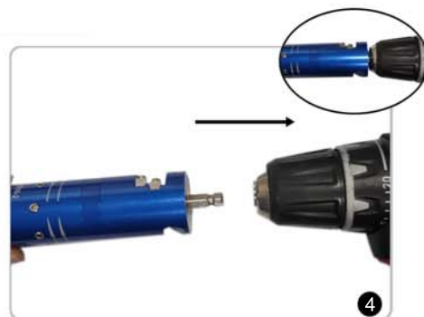
Attach the trimming tool to power drill.
