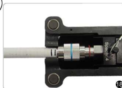
18 Make sure the connector nut is lined up against spacer 4 to prevent damage to the O-ring during compression.
